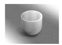
Crucible TK-36 can be used to heat tratement and chemical reacting of small amounts of substances. Designed to use with crucible stools or holders because of spherical bottom. Manufacturing in high pressure Ceramic Injection Molding technology ensures keeping accuracy of shape and narrow dimensional tolerances.
