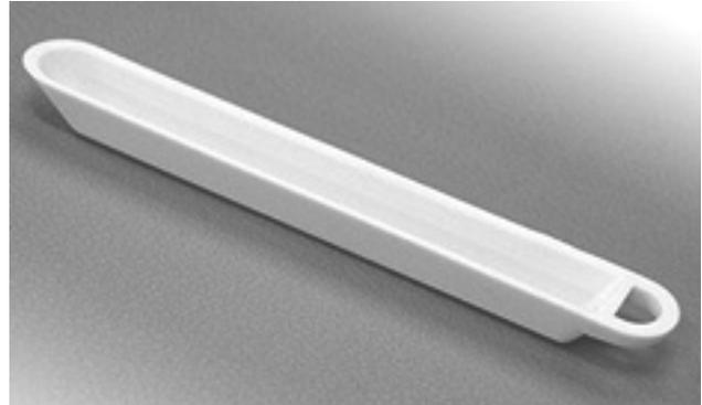
Combustion Boat L-101 can be used to heat treatment and chemical reacting of small amounts of substances. Elongated shape and flat bottom facilitates locating in furnaces or on shelves. Holder enables moving a hot boat. Manufacturing in high pressure Ceramic Injection Moulding technology ensures keeping accuracy of shape and narrow dimensional tolerances.
